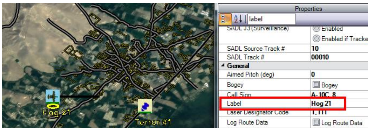
Figure 11: Add a Label (using the Property Grid) to a Site, Platform or Waypoint
